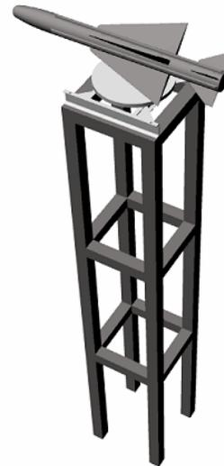
Fig. 2. Pylon for RCS measurements with a hypothetical target. Top view. The width of the pylon is 1.4 m and its height is 7.95 m. A structure that houses a turntable is mounted atop the pylon. The height of this structure is 0.2 m. The target, a generic missile, has a length of 3.15 m. It is included in the figure for scale. The braces holding the missile in place are hidden from view by its body.
