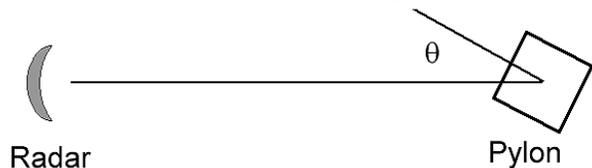
Fig. 3. Relative orientation of the pylon with respect to the radar.  $\theta$  is the aspect angle.
