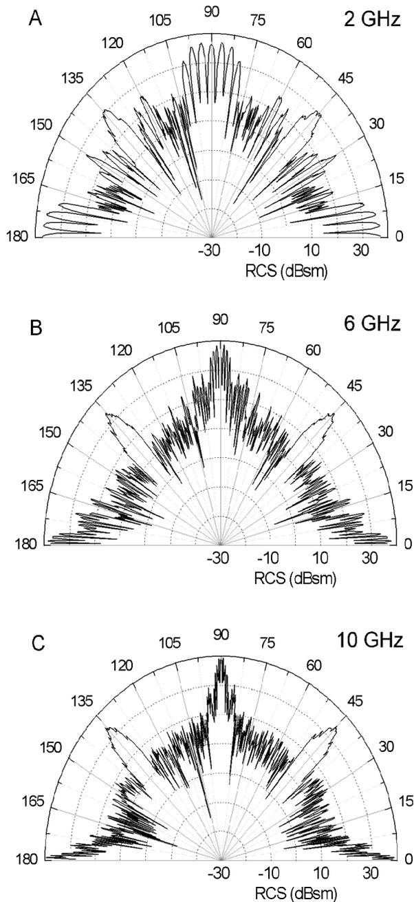
Fig. 4. Polar plots of the simulated RCS of the model of the pylon versus the aspect angle. Simulations performed at 2, 6 and 10 GHz are represented in the panels A, B and C, respectively. At 0°, 90° and 180°, the line-of-sight on the radar is perpendicular to the side of the pylon. At 45° and 135°, the line-of-sight of the radar is aligned with the corners of the pylon. RCS values were simulated at intervals of 0.25°.
